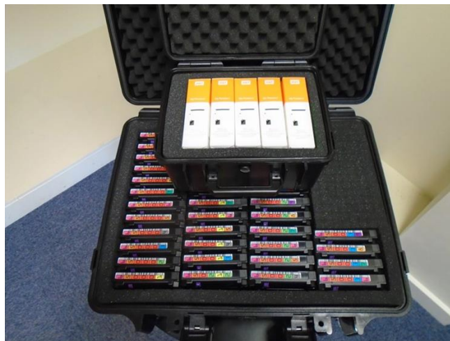
Remastered seismic data representing 39 surveys acquired over 30 years, transcribed on to 40 x 4TB 3590JC magnetic tapes for archiving and 5 High density USB disks for ready access
