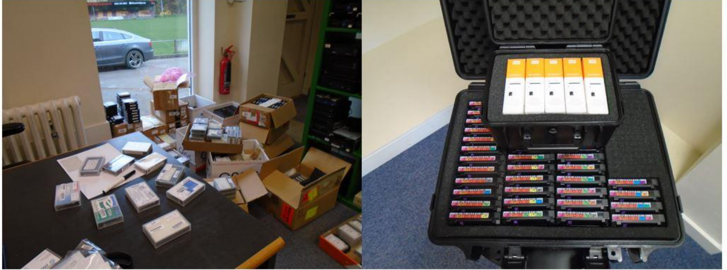
Remastered seismic data representing 39 surveys acquired over 30 years, transcribed to 40 x 4TB 3590JC magnetic tapes for archiving and 5 x USB HDD's for ready access
