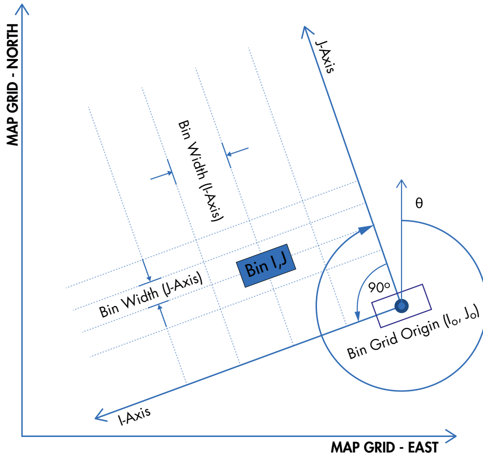
Figure 2: I-axis is 90 degrees counter-clockwise from the J-axis when viewed from above the plane of the two bin grid axes.
